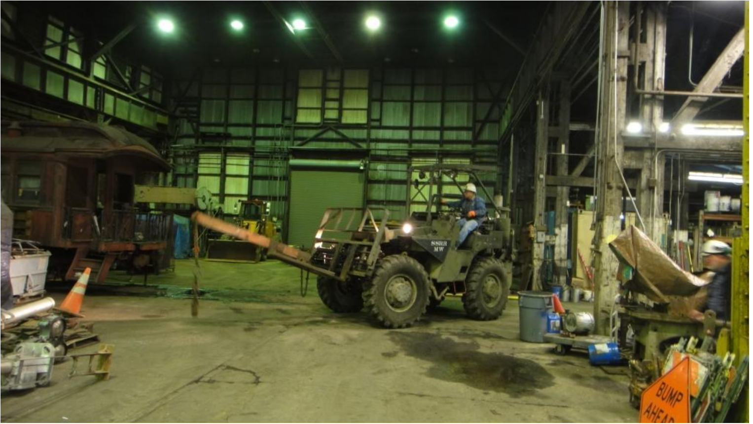
Mike H. grabs the "stinger (for lifting rail) with Big Green
